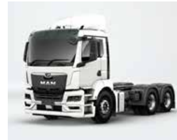
CAB NN: THE PRACTICAL ONE (narrow, medium length, standard height)
