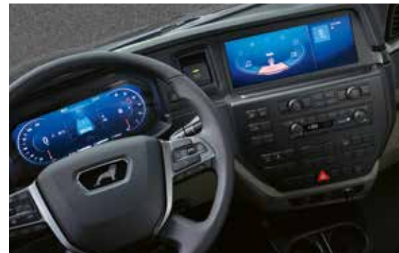
Infotainment system with 12.3-inch display and control system below the secondary display*
