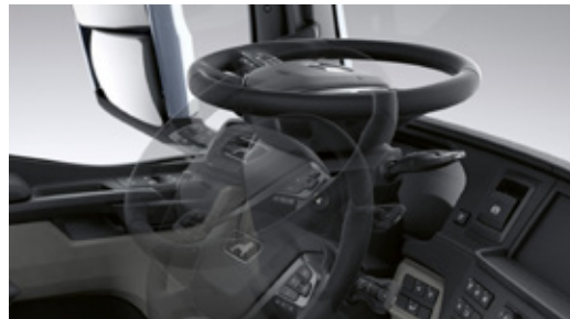
Passenger car like steering adjustability. A considerably steeper steering wheel angle is possible, similar to that in a passenger car.
