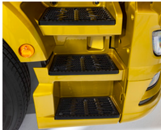
New arrangement of steps: The steps are arranged like stairs, so that when the driver exits the cab he is able to see a part of the lowest step.
